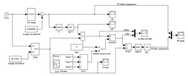
Fig. 4. Matlab Simulink PF increasing simplified model
