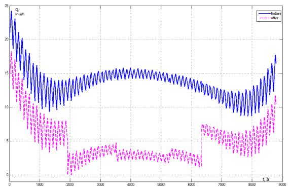
Fig. 7. Calculated reactive electrical energy in MatLab Simulink by ActC full method
