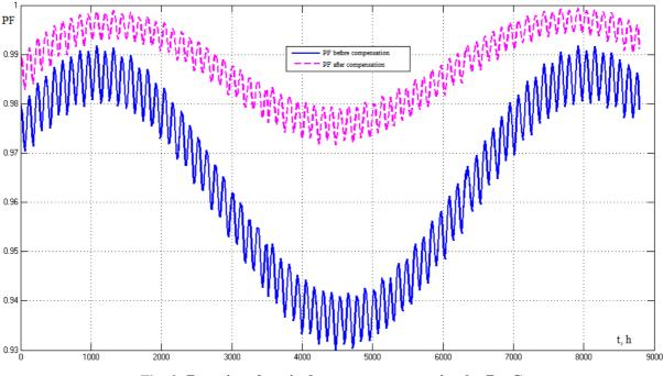
Fig. 3. Reactive electrical power compensation by PasC
