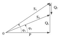
Fig. 1. Opposite character reactive electrical power connection, vector diagram and PF change
